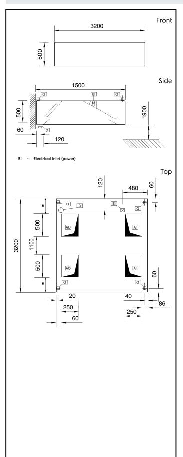
**Electric** Supply voltage: 641262 (STPF1532) 220 V/1N ph/50 Hz **Total Watts:** 0.24 kW Capacity: Supply capacity: 3180 m<sup>3</sup>/h **Key Information:** External dimensions, Width: 3200 mm External dimensions, Depth: 1500 mm External dimensions, Height: 500 mm Net weight: 203 kg Air Emission:
